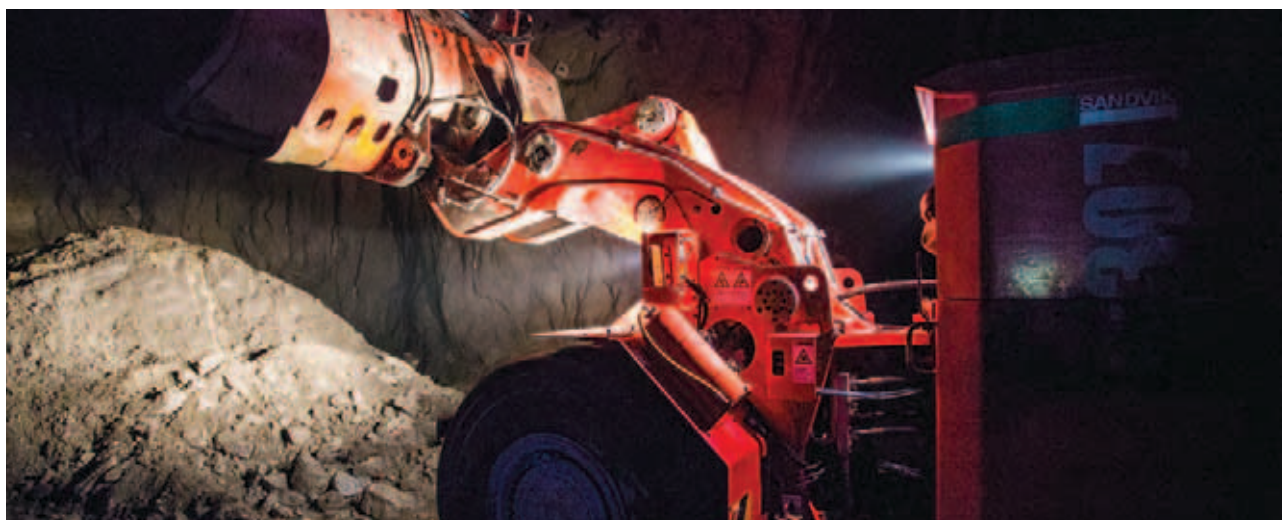
ORE MUCKING UNDERGROUND, MARULA
