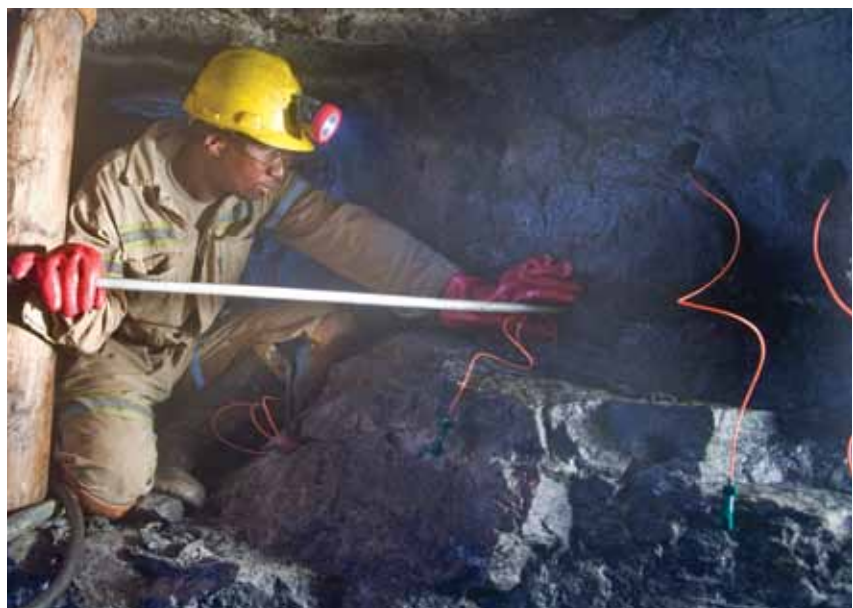
Charging up in a ledging section at BRPM
