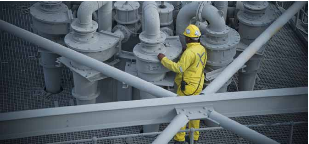
Safety representative inspecting secondary mill cyclone cluster
