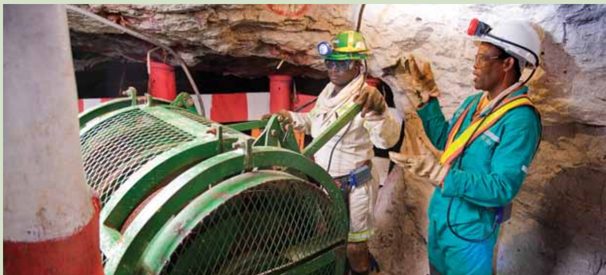
An instructor trains a new winchdriver in the operation of a scraper winch installation
