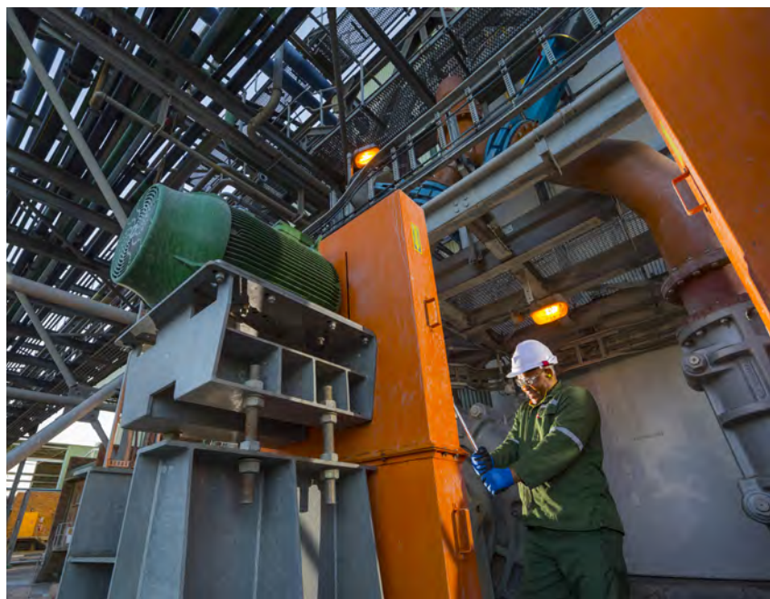
New flotation pumps at the BRPM concentrator
