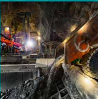
Tipping of ore into an ore pass (OPC4) at 600 level
