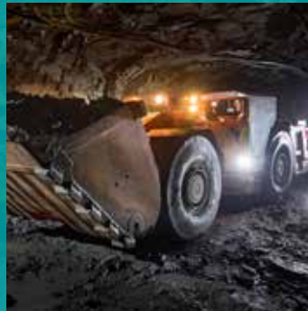
LHD tramping ore on 600 level
