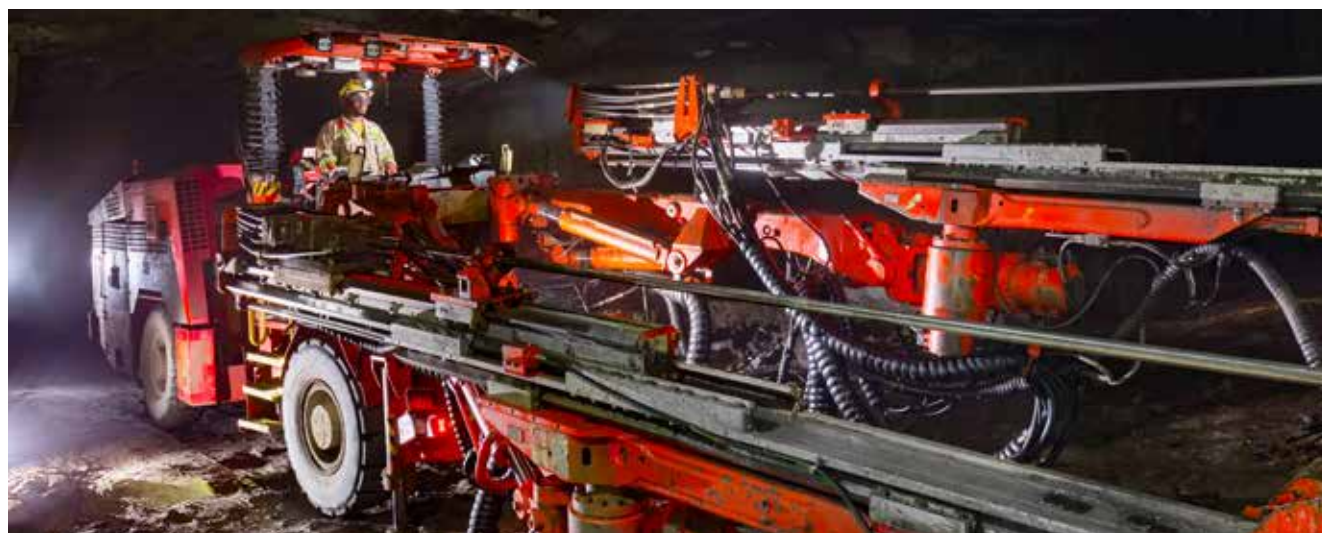
Double boom drillrig, Styldrift I shaft, 600 Level
