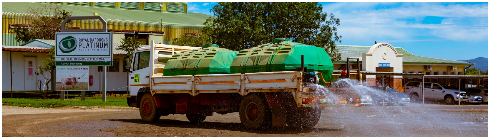
The water used for dust suppression in our operations and the surrounding communities is drawn from water recycled in our closed loop system
