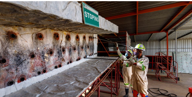
A stoping face mock-up in the BRPM training centre
