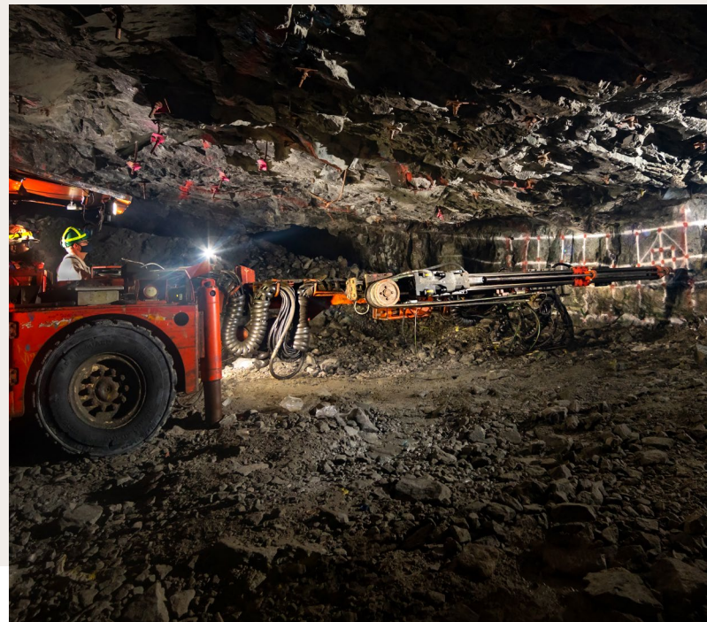
Mechanised stope face drilling on 600 Level at Styldrift
