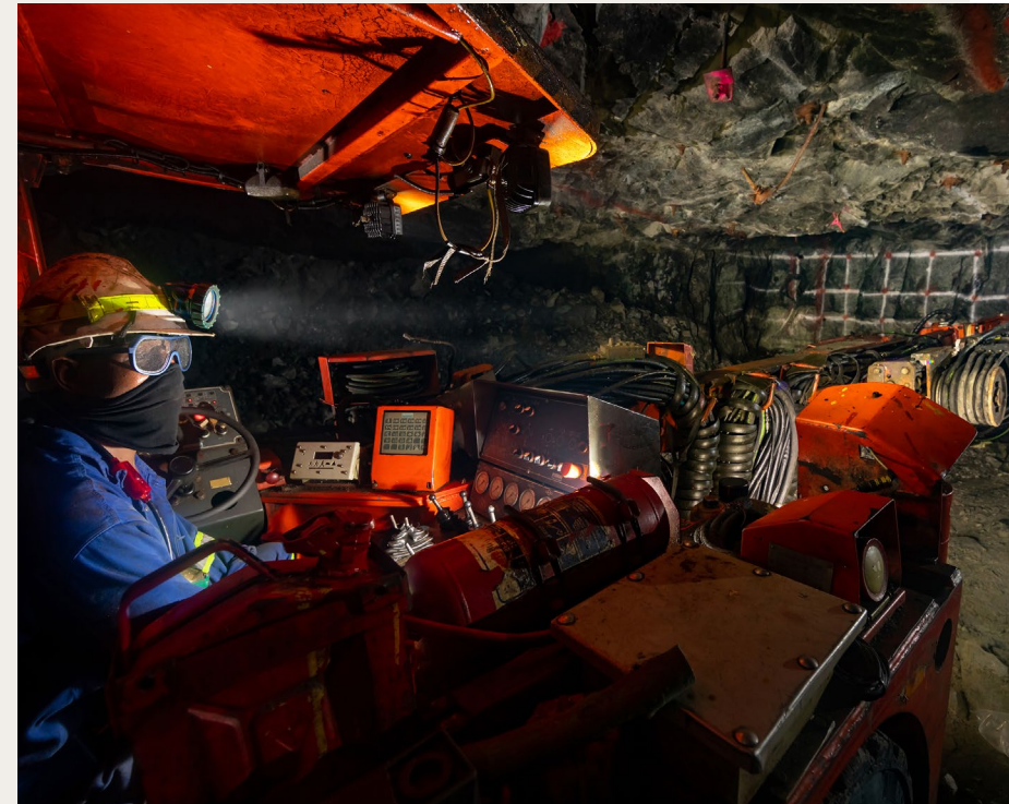
Face drilling of a stoping bord on 600 Level at Styldrift
